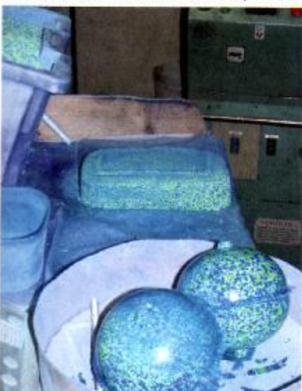
The melamine before it is put into the moulder at the back, and after this process, in the foreground. As you can see, there are still 'lugs' on either end.
