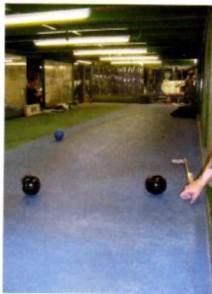
The test table used to ensure the set run identically and that they comply with the minimum bias of the World Bowls Board
